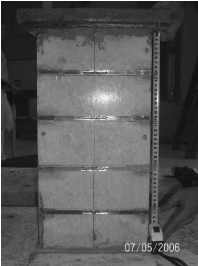
Figure 21.14 Experiment setup in the functional test: The silver strips are the CRM gages being deployed.
