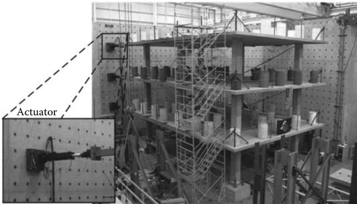
Figure 21.16 Three-story reinforced concrete building structure in the full-scale experiment.
